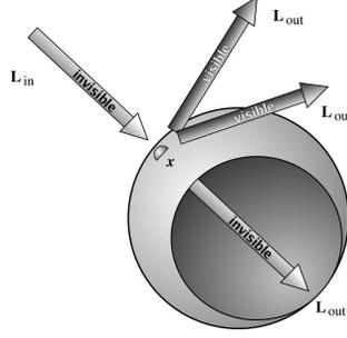
**Figure 3.** Incident invisible radiance  $\mathbf{L}_{in}$  strikes a point  $x$  on a sphere (cut-away view). The surface transmits invisible light while reflecting visible light.
