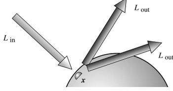
**Figure 2.** Incident radiance  $L_{\text{in}}$  strikes a point  $x$  on the surface and reflects with radiance  $L_{\text{out}}$  in directions  $\omega_{\text{out}}$
